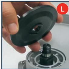
Fit the new disc, ensuring that the disc is correctly located on the inner flange.
