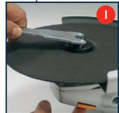
spindle lock engages and locks the spindle. Use the pin wrench (11) to unscrew the outer flange (13). Note that this flange unscrews anticlockwise. (Fig. I)
