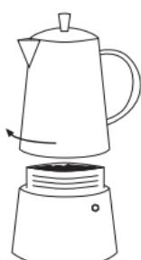
3. Place the funnel filter back inside, fill it with espresso coffee powder and smooth the powder down. Do not press the powder down hard into the funnel filter!
