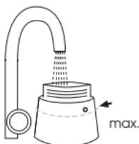
2. Fill the lower part of the espresso maker with enough water so that the water level rises to just below the safety valve at the most. Under **no** circumstances must the safety valve ever be under water.
