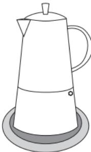
5. Place the espresso maker on a heat source and heat up. To avoid overboiling and to maintain your espresso maker in good condition, we recommend that you do not allow the espresso to reach too high a temperature. The espresso coffee will rise with the slightest development of steam and will begin to gurgle quietly into the upper receptacle. Remove the espresso maker from the heat source immediately as soon as this gurgling ceases.
