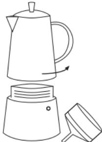
1. Unscrew the espresso maker by taking hold of the upper and lower parts and turning (one part) anti-clockwise. Remove the funnel filter.
