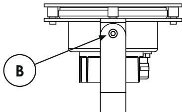
1. Untighten the lateral screw "B", rotate the body of the unit towards desired direction and tighten the knobs.
