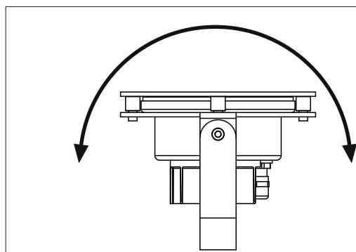
2. Rotate the body of the unit towards desired direction and tighten the screw "B".
