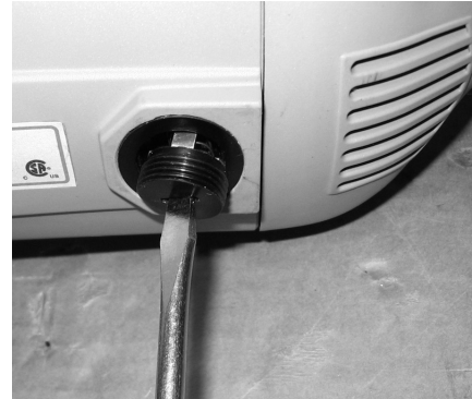
Inspecting the Carbon Brushes (50)
