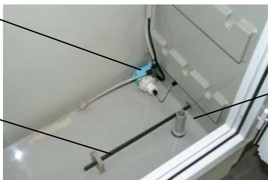
Detail of overflow inside cabinet for discharge of water (in foreground) and recycle pump (in background). In between is the heating resistance.
