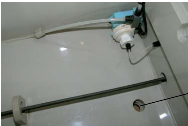
Detail of overflow tube for discharge of water and of re-circulation pump.
