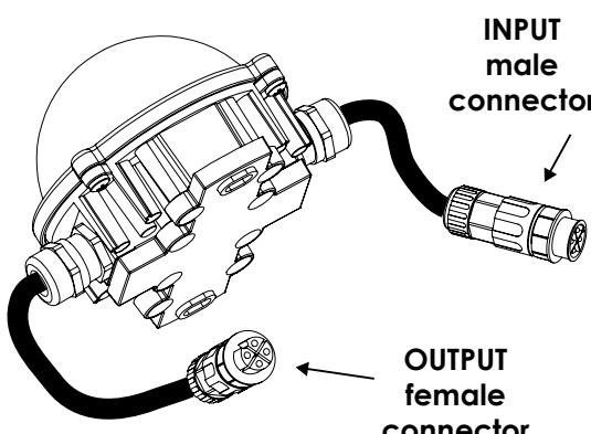
The unit is fitted with IP68 connectors for the connection of the of the main supply and of the DMX signal, as shown in the pictures.
