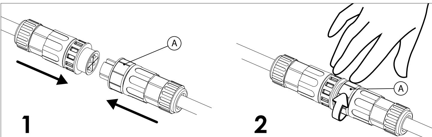
Plug the connectors by screwing the ring "A" by hand.
