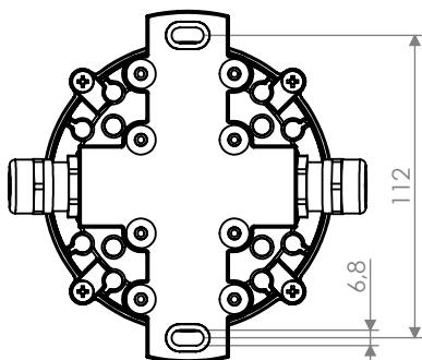
Use the two Ø6.8 holes (0.26") on the box in order to fix the device
