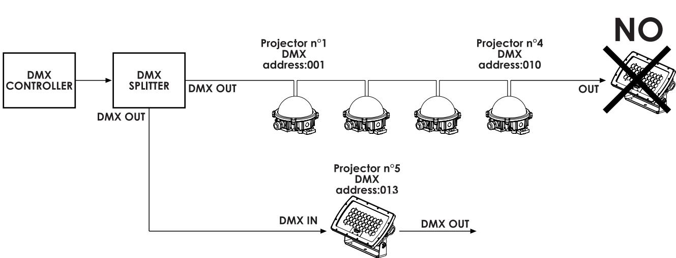
The following picture shows an example of installation with DMX control and electronic driver.
