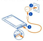
2 When the battery is full, unplug the charger from the phone, then from the wall outlet.
