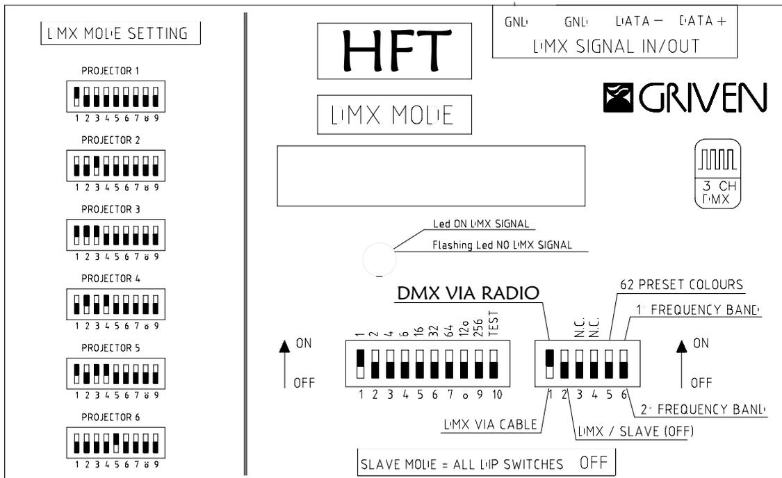
The dip switches have the same function as when the unit operates in DMX/SLAVE mode (see 4.4 DMX/SLAVE mode), apart from dip switches no. 1 and 6 of the second group:
