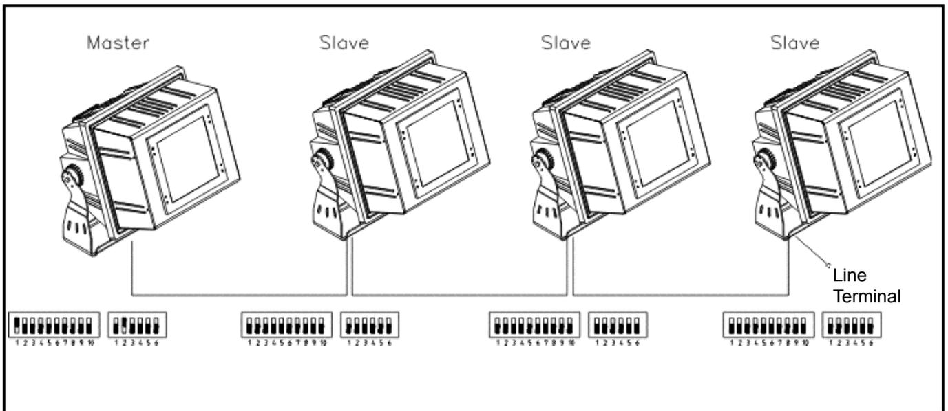
The DMX specifications require a 100-120 ohm terminal resistor, which must be fitted between the DATA+ and DATA- Pins in the last unit of the DMX line. For each DMX line select Master mode or DMX mode, but not both of them, because in this last case the electrical line may be damaged.
