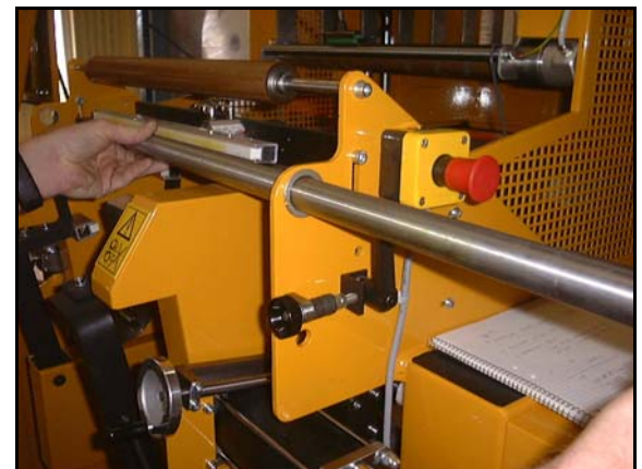
Fig. 44 Loosen the bar and withdraw the axle
