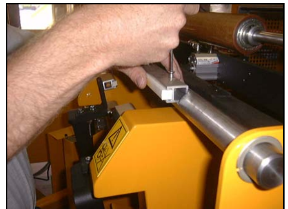
Fig. 43 Loosen the screws holding the bar
