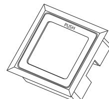
**WARNING: IN ORDER TO BE ABLE TO CLOSE THE SPOTLIGHT AGAIN, ONCE THE COVER IS OPENED BY PRESSING ON THE “PUSH” SIGN, IT IS MANDATORY THAT THE COVER BE OPENED WIDE TO TRIGGER THE SPRING SUPPORT AND MAKE IT SETTLE IN ITS CORRECT POSITION.**
