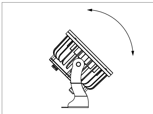
2. Rotate the bodies of the unit towards desired direction and tighten the screw “2”.
