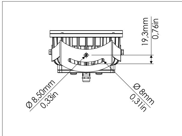
Use the holes Ø8.5 (1/4") in the bracket to fix the unit.
