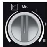
The pump speed is set with the knob.
