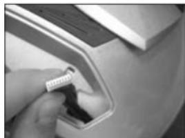
3) Slip on the connector with 8 poles between the EPS and the shell in order that the cable comes out from the apposite slit. Connect the key pad with the Connector and place it in its seating on the shell .
