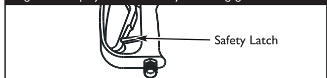
Figure 7 — Spray Gun with Safety Latch Engaged
