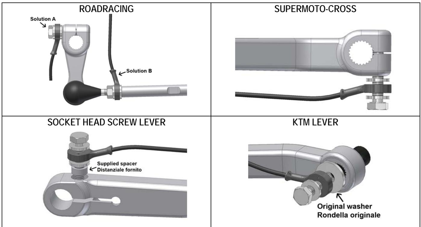
Please Note: In case of assembly on levers complete with a socket head screw, insert the spacer supplied with the kit to balance the original seat height.
