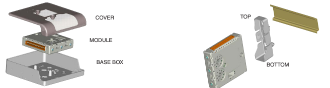
FIGURE 1: MODULE MOUNTING METHODS
