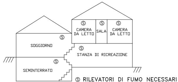
Split level arrangement. Smoke detectors are required where shown. Smoke detectors are optional if door is not provided between living and recreation rooms. DISPOSIZIONE NEI LIVELLI SEPARATI. I RILEVATORI DI FUMO SONO NECESSARI DOVE MOSTRATO. I RILEVATORI DI FUMO SONO OPZIONALI SE NON C'È PORTA TRA IL SOGGIORNO E LA STANZA DI RICREAZIONE
