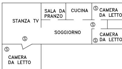
(B) IN UNITÀ ABITATIVE FAMILIARI CON PIÙ DI UN'AREA NOTTE, SI DOVREBBE FORNIRE UN RILEVATORE DI FUMO IN OGNI AREA NOTTE IN AGGIUNTA AI RILEVATORI RICHIESTE NELLA CAMERE DA LETTO.
