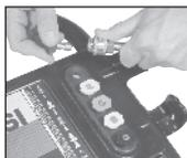
**⚠ WARNING** Risk of Flying Object could cause risk of serious injury. **Ensure nozzle is completely inserted in QC socket, and QC snap ring is fully engaged (forward) before squeezing gun trigger.**
