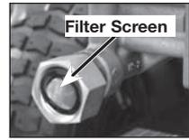
2. **Clean filter** by flushing it with water on both sides.
