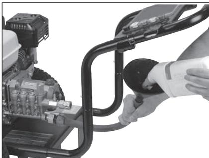
5. Pull engine starter rope slowly several times until antifreeze comes out of high pressure hose connection of pump.
