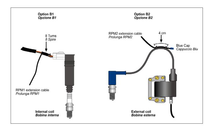
**Attention!** Never connect the RPM reading wire directly to the coil wire to prevent any inadequate voltage irreparably damaging the instrument.
