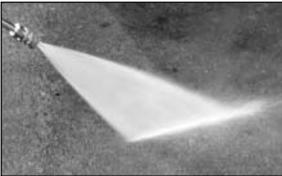
**25° nozzle - Green.** This nozzle delivers a 25 degree spray pattern for intense cleaning of larger areas. This nozzle should only be used on areas that can withstand the pressure from this nozzle.
