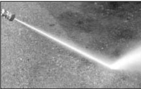
**0° nozzle - Red.** This nozzle delivers a pinpoint stream and is extremely powerful. It covers a very small area of cleaning. This nozzle should only be used on surfaces that can withstand this high pressure such as metal or concrete. Do not use on wood.
