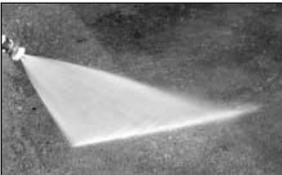
**40° nozzle - White.** This nozzle delivers a 40 degree spray pattern and a less powerful stream of water. It covers a wide area of cleaning. This nozzle should be used for most general cleaning jobs.
