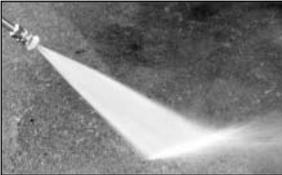
**15° nozzle - Yellow.** This nozzle delivers a powerful 15 degree spray pattern for intense cleaning of small areas. This nozzle should only be used on areas that can withstand the high pressure from this nozzle.
