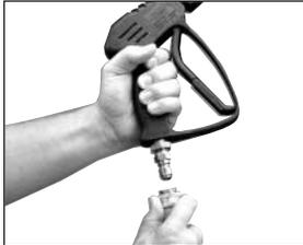
5. Assemble grommet kit and quick-connect nozzles as described in instructions supplied.
