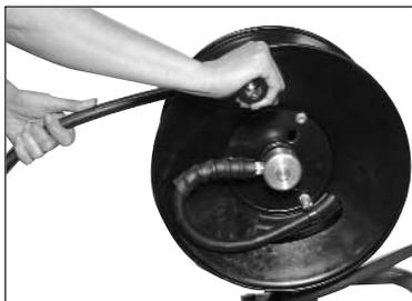
9. Attach hose reel inlet to high pressure pump.
