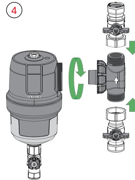
Unscrew T piece from filter body and assemble isolation valves in closed position
