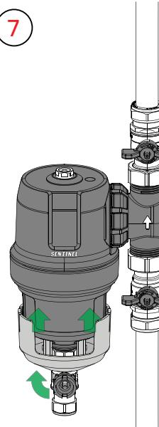
Close drain valve and re-engage magnetic tray
