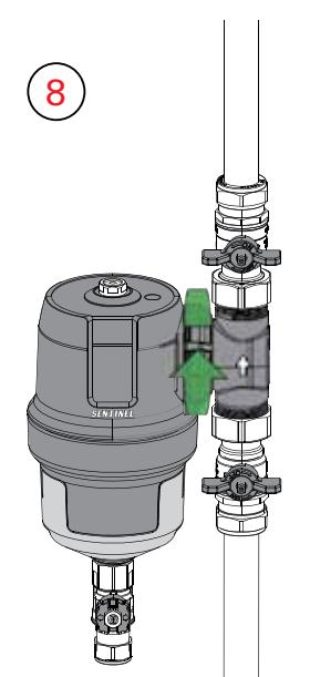
Lock filter to T piece using collar
