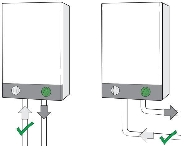
Position filter on return pipe close to boiler
