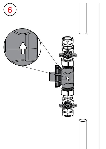
Fix isolation valve assembly into cut pipe. Ensure the direction of flow matches the direction arrow on the filter
