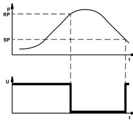
Signal "off" with falling pressure
