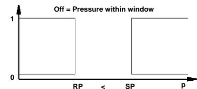
Std = Standard mode, switching and reset points adjustable
