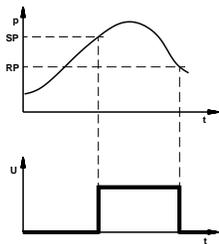
Signal "on" with falling pressure
