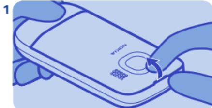
Switch the phone off. Lift and remove the back cover.
