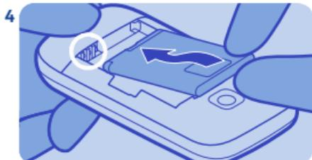
Line up the battery contacts, then push the battery in.
