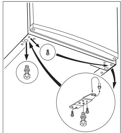
6. Unscrew the top door hinge pin of the appliance then screw it back on the other side.
