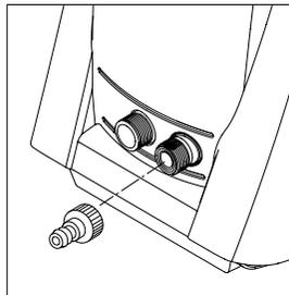
1. Screw the quick coupling (16) tight on to the water inlet (2).
