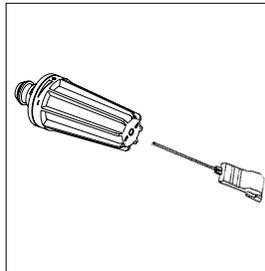
A clogging up in the nozzle causes a pump pressure which is too high. This is why cleaning is required immediately.
