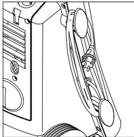
To avoid accidents, the electric cable and the high pressure hose should always be wound carefully up.
