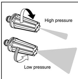
The pressure can be regulated on the TORNADO® PR nozzle.
