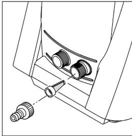
Clean the water inlet filter regularly once a month or more frequently according to use. Carefully loosen the filter with a pair of pliers and clean it. Check that it is intact before re-mounting it.
