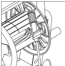
The high pressure washer comes in two models: A) with hook for storage of high pressure hose (14) - B) with a hose reel (13), where the hose is pushed into the reel and afterwards wound up.
