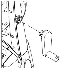
1. Click the hose reel handle on to the trolley handle (no screws).
