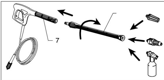
1. Push the spray lance (6) into the spray gun (7) and screw it on.
