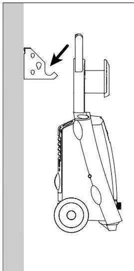
If mounting a special wall hook (not standard), the pressure washer can be used as a stationary solution meaning that it can be operated while hanging on the wall.
