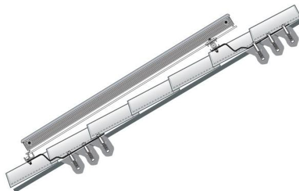
Assembling on roof with tiles you can use special frame. These are available for 1,2 o 3 panels HIT and HIS or for 1 or 2 panels HITX, HISX
