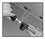
**Step 3** Insert upper handle into the lower handle by twisting together.
