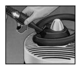
**Step 5** Tighten lock collar to assemble by twisting counter clockwise.
