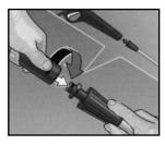
**Step 6** Insert pressure washer wand into upper lhandle. Push wand down over upper handle and twist clock-wise 1/4 turn into locked position.
