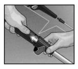
**Step 7** Turn locking collar clock-wise over pressure washer wand until tight.
