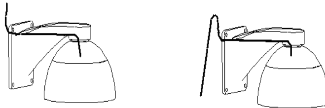
Wrong wiring: from upper to nether
