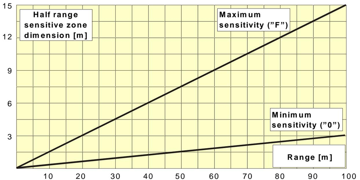
Figure 3a **Vertical** plane Half range sensitive zone dimension for CORAL 100 (free space)
