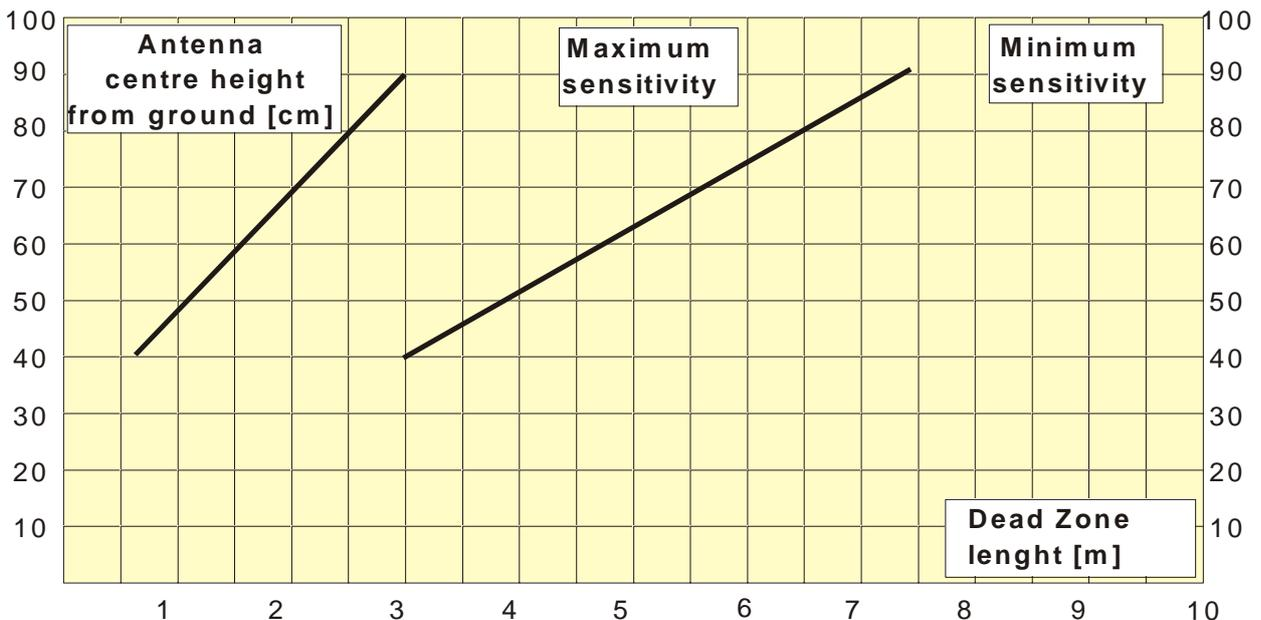
Figure 5 CORAL-PLUS 100 Dead zone length near the equipment versus antenna centre height from ground.
