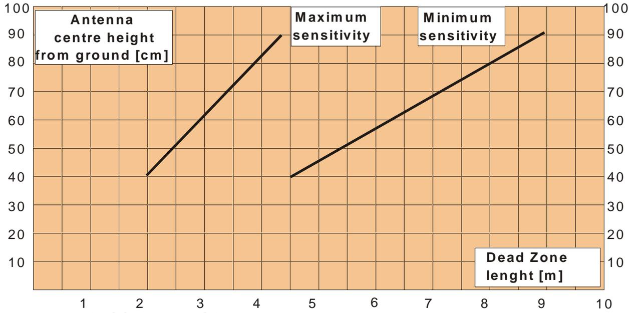
Figure 6 CORAL-PLUS 220: Dead zone length near the equipment versus antenna centre height from ground.
