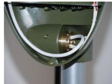
6. Finally close the MW head using the 6 screws to fix the radome.
