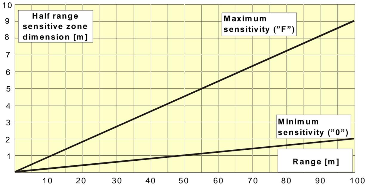
Figure 3 **Horizontal** plane Half range sensitive zone dimension for CORAL-PLUS 100 (free space)
