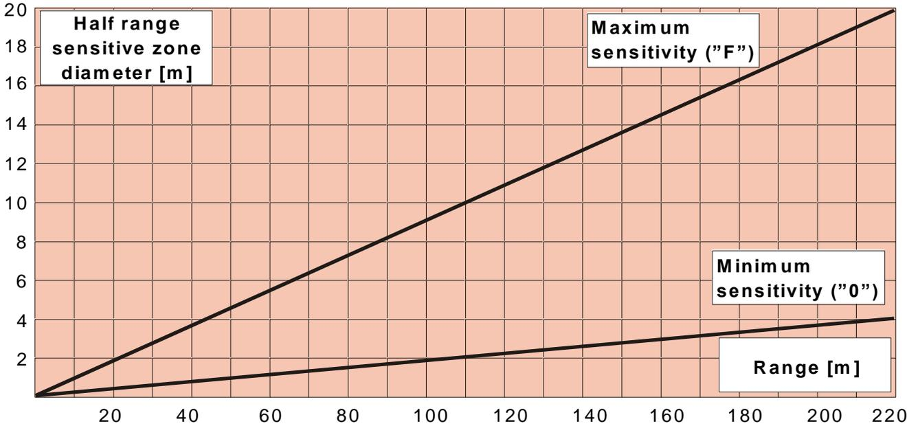
Figure 4 Half range sensitive zone diameter for CORAL-PLUS 220 (free space)
