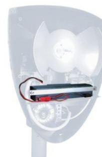
3. Connect the “fastons” to the battery and remember to respect the polarity that means, red wire (Terminal 1 of MS2) to the positive of the battery and black wire (Terminal 2 MS2) to the negative of the battery.
