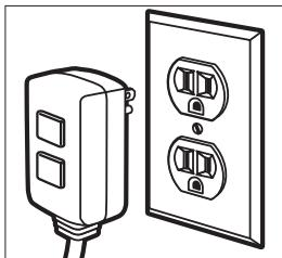
**Step 1** Plug the Ground Fault Circuit Interrupter (GFCI) into a working outlet.
