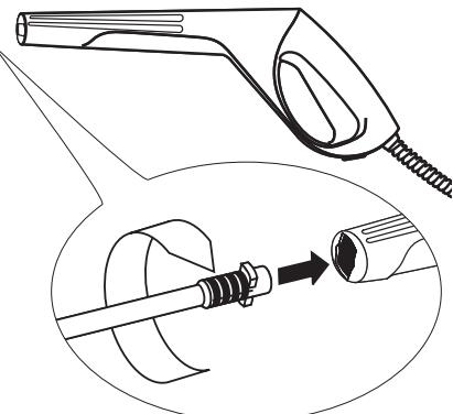
**Step 2** Insert the spray wand of your choice into the trigger gun. Push in and turn clockwise to lock spray wand in place.
