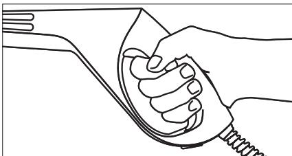
**Step 3** Turn on the pressure washer. Pull trigger to operate unit: Liquid detergent is drawn into the unit and mixed with water. Apply detergent to work area. Do not allow detergent to dry on surface.
