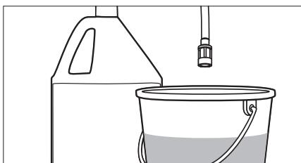
**Step 2** Fill a container with Karcher detergent. Place the filter end of detergent suction tube into the container.
