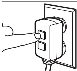
**Step 2** Press "TEST", then press "RESET" to assure proper connection to power.
