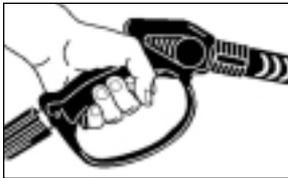
**Step 2** Press trigger to release water pressure.
