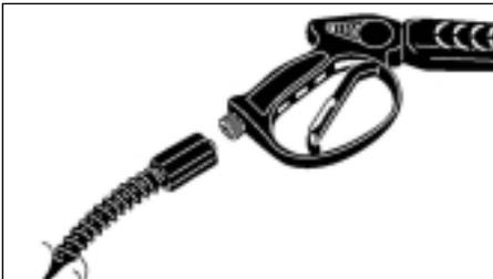
**Step 5** Attach high pressure hose to trigger gun.
