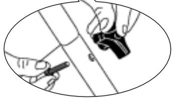
**Step 3** Insert the handle into the frame. Align holes, insert bolt, and tighten with knob.
