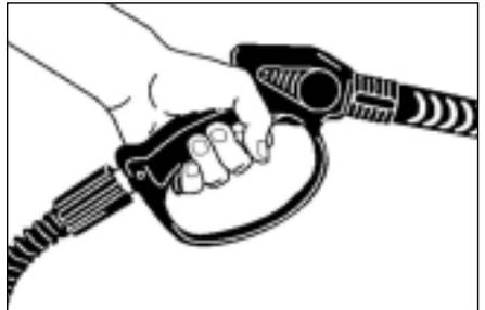
**Step 6** Trigger the gun to eliminate trapped air, wait for a steady flow of water to emerge from the spray nozzle.
