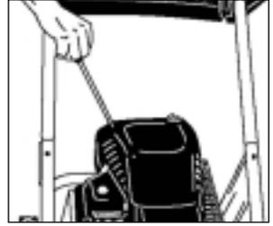
**Step 9** Pull the starter handle. If the engine fails to start after 3 pulls squeeze the trigger gun to release pressure, and repeat step 9.
