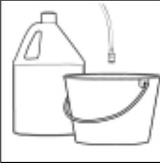
**Step 1** Remove detergent suction tube from container and insert into one gallon of fresh water. Siphon water at low pressure for one minute.
