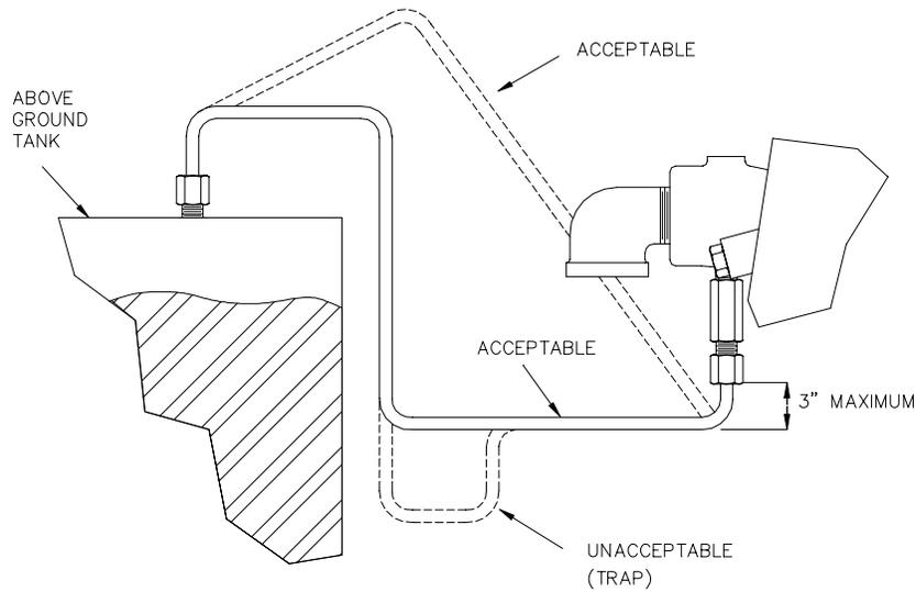
**NOTE:** *Tubing can be piped to any available opening on top of tank. Use reducer bushings as required.*
