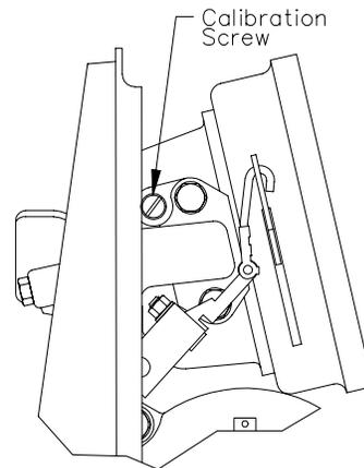
Replace the cap screw (old style only). Deliver about 1/2 gallon through the meter before resetting to zero and retesting. Allow a ten second drain period each time the test measure is emptied to assure accurate measure. Adjust and retest until register is zeroed at desired flow.
