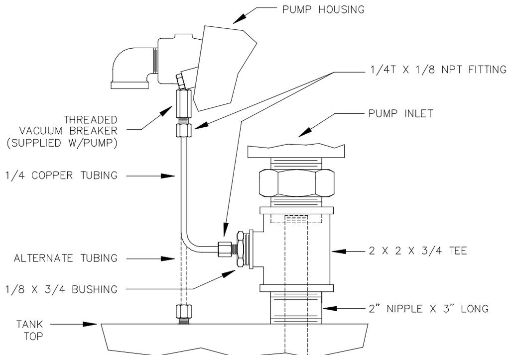
**NOTE:** *Tubing can be piped to any available opening on top of tank. Use reducer bushings as required.*
