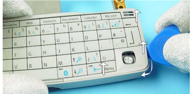
26.) Unlock the hooks along the edge of the Qwerty Keypad as shown.
