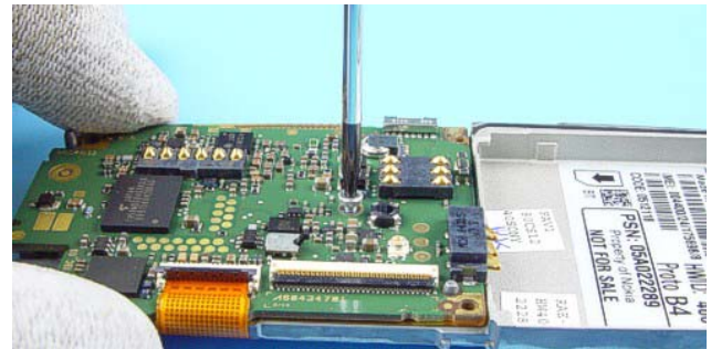
44.) Unscrew the Torx Plus® size 6 screw.
