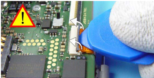
43.) Unlock the QWERTY flex connector with SRT-6 carefully.
