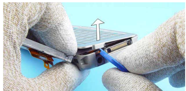
24.) Place the SRT-6 between Qwerty Keypad and the DC-Jack and lift the Qwerty Keypad carefully.
