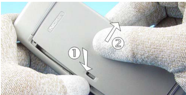
3.) Press down the Latch and open the Battery Cover .
