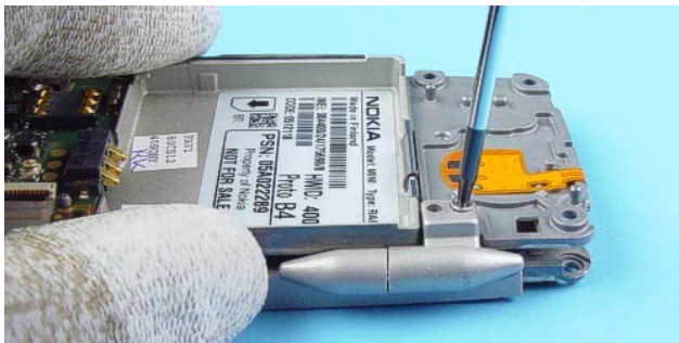
41.) Unscrew the Torx Plus® size 6 screw.
