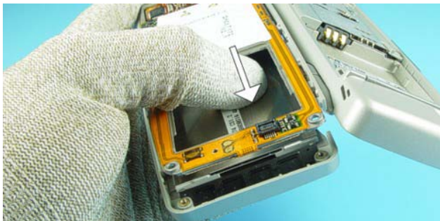
21.) Press out the C-Cover Assy carefully.
