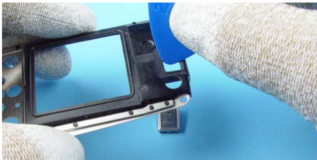
13.) Push out the Speaker with SRT-6.
