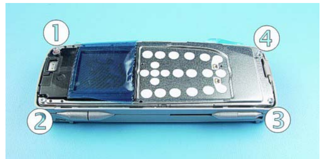
8.) Unscrew the four, Torx Plus® size 6 screws in the shown order. Always use new screws when re-assembling! For assembly, reverse the order and use a Torx Plus® size 6 driver with a torque setting of 25Ncm.
