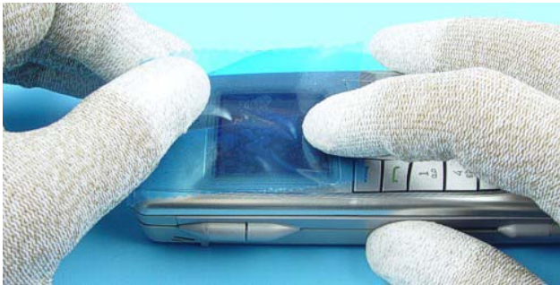
1.) Protect the window with a film.
