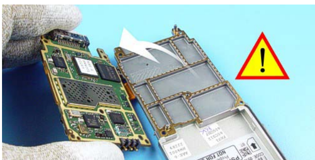
45.) Turn the Engine Module. Take care of the RF Gasket.
