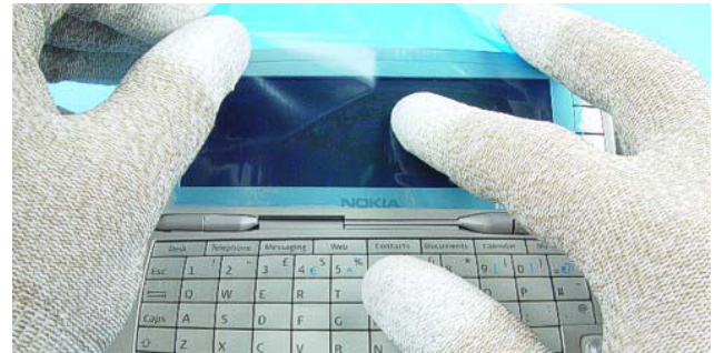
2.) Fit protective film to the LCD Module .
