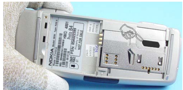
4.) Be sure that the battery is removed and then continue with disassembly. Note to put back the Sealing Tape after the re-assembly.
