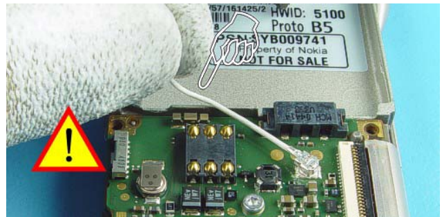
37.) Do not pull up on the cable.
