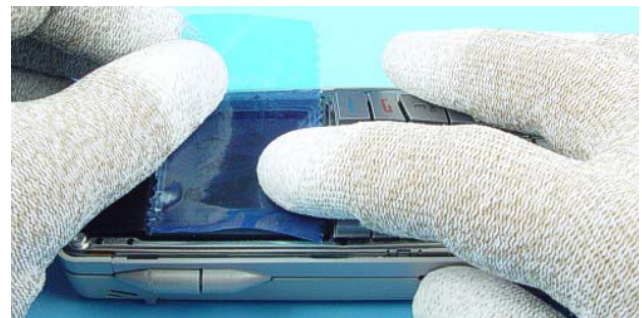
6.) Protect the LCD Module with a film.
