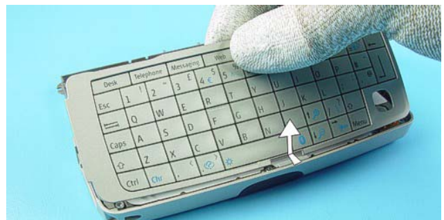
28.) Now, the Qwerty Keypad can be removed.
