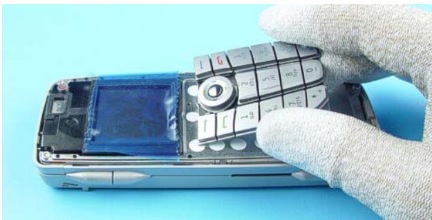
7.) Remove the Keypad . Note the guide openings on the UI Shield Assy when assembling the Keypad .
