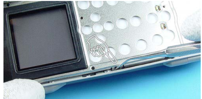
10.) Open the flap carefully by using the dental tool.
