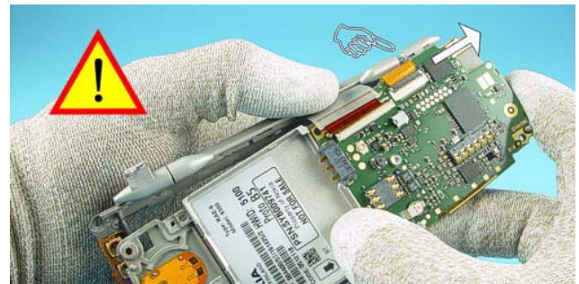
42.) Separate the 1CP QWERTY Flex Module from Chassis.
