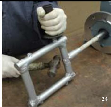
*Disassemble the pump shaft (17), only if it is deteriorated or if the motor bearings need replacing, proceed as follow:*
