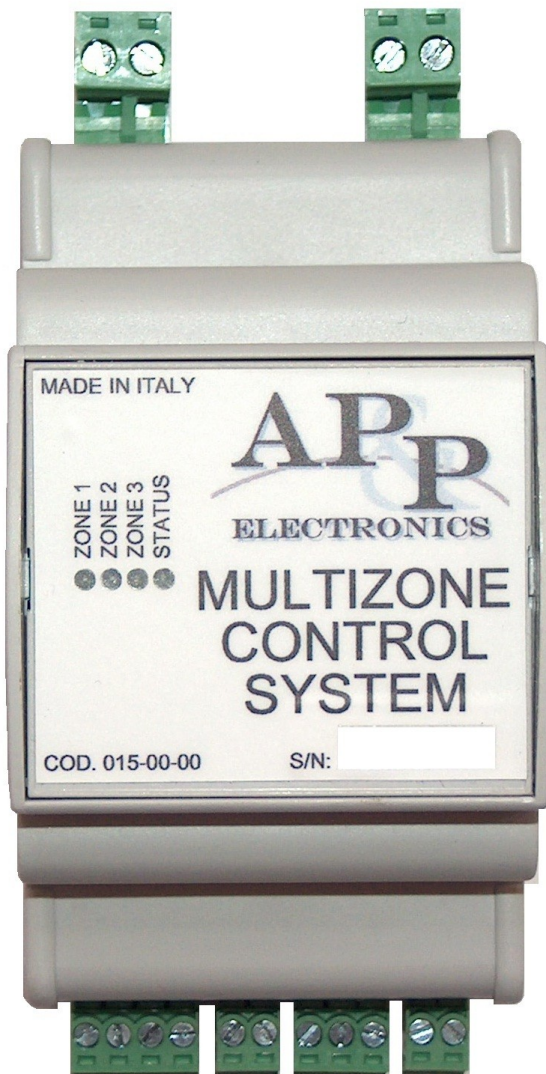
Figura 1: Multizone Control System
