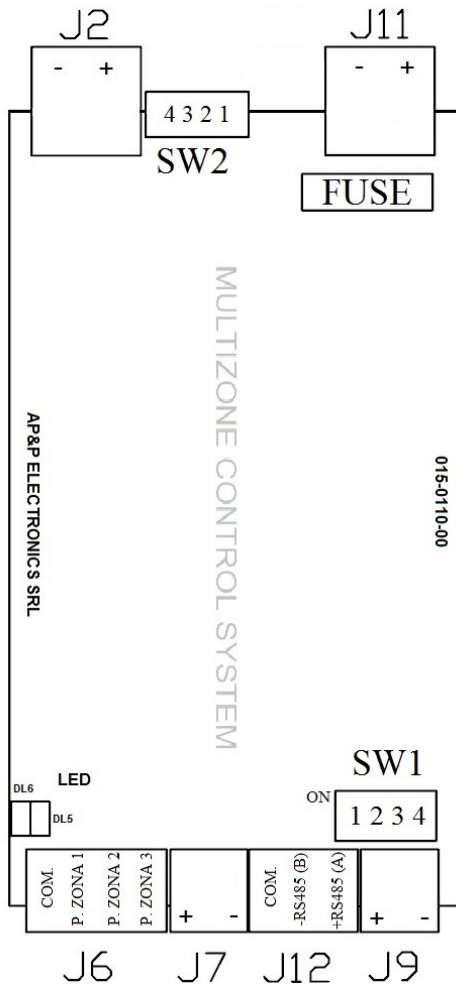
Figura 2: Layout centralina Multizone Control System
