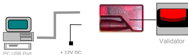
Figure 2 - Connecting DA2 to a NV10 and PC for upgrading
