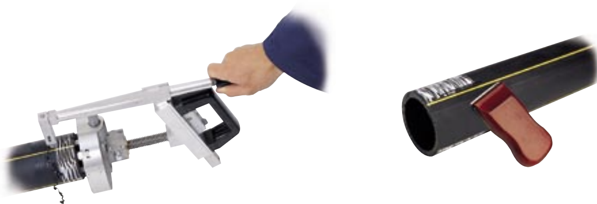
Cleaning the pipe with mechanical scraper code 3855 and hand scraper code 3856
