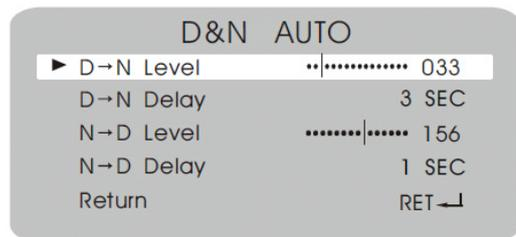
**D -> N Level:** camera sensitivity level from color to B/W mode.
