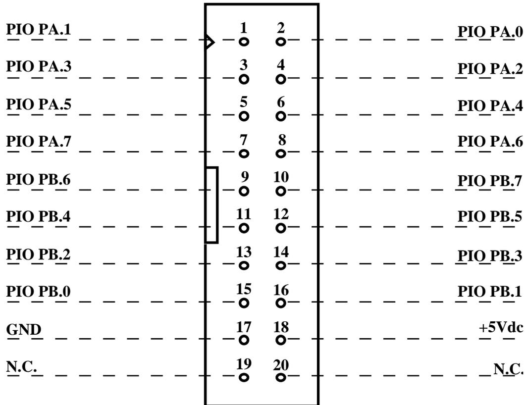
FIGURA 16: CN5 - CONNETTORE PER I/O DEL PIO
