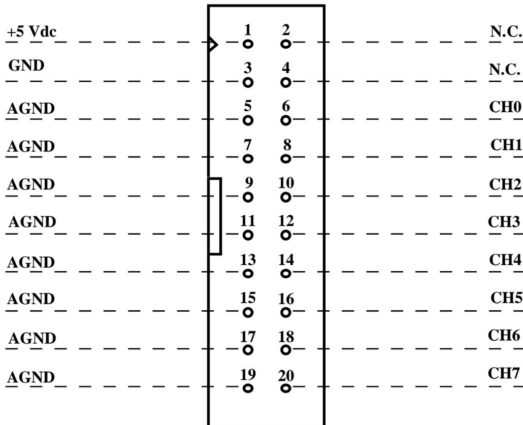
FIGURA 18: CN5 - CONNETTORE PER INGRESSI A/D CONVERTER
