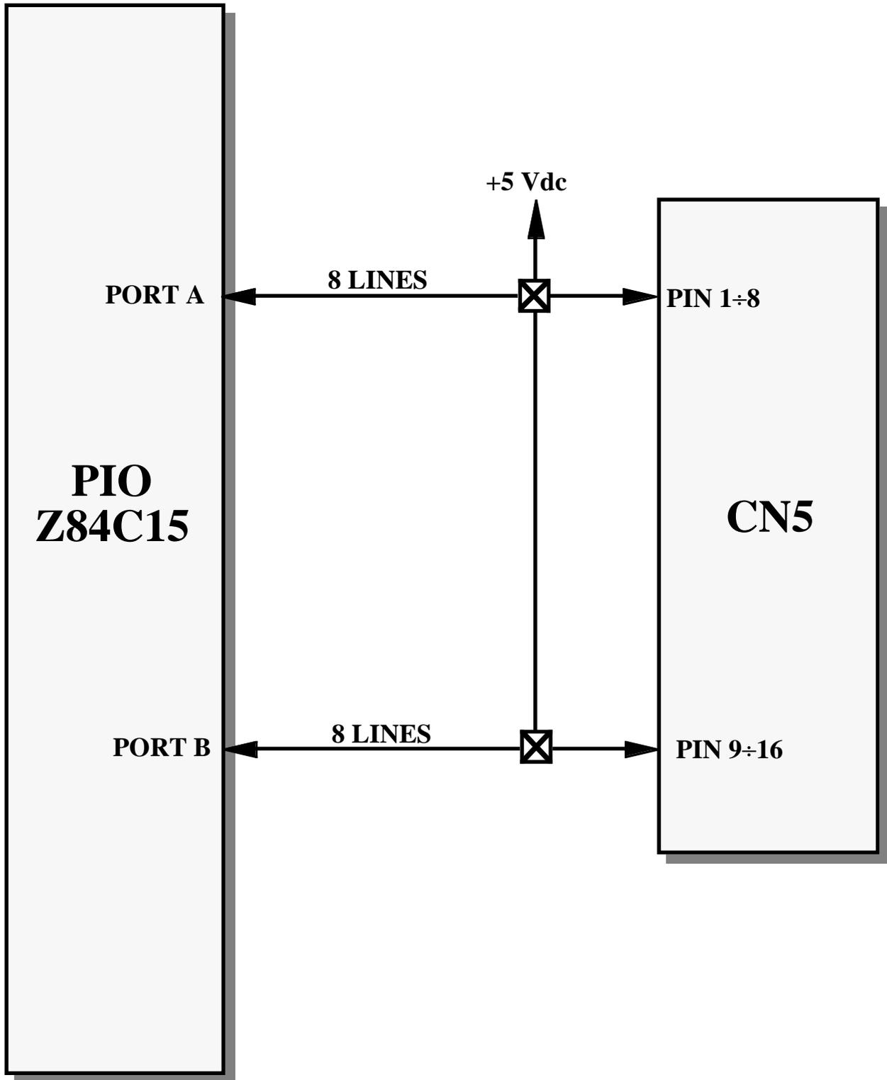
FIGURA 17: SCHEMA DEL COLLEGAMENTO LINEE DI I/O DEL PIO
