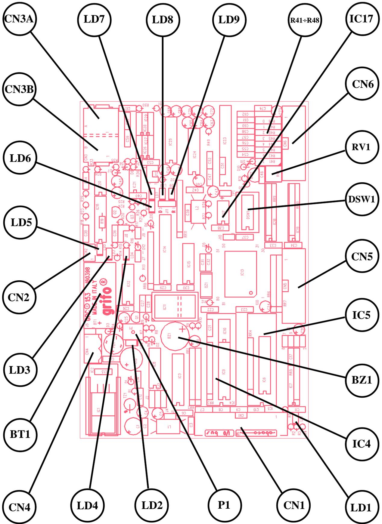
FIGURA 20: DISPOSIZIONE CONNETTORI, MEMORIE, DIP SWITCH ETC.
