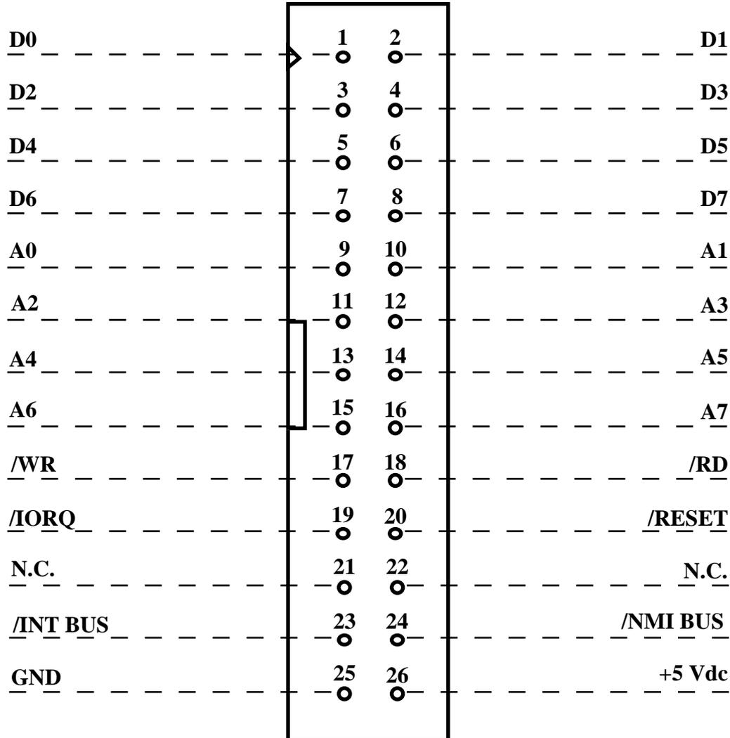
**FIGURA 4: CN1 - CONNETTORE PER ABACO® I/O BUS**
