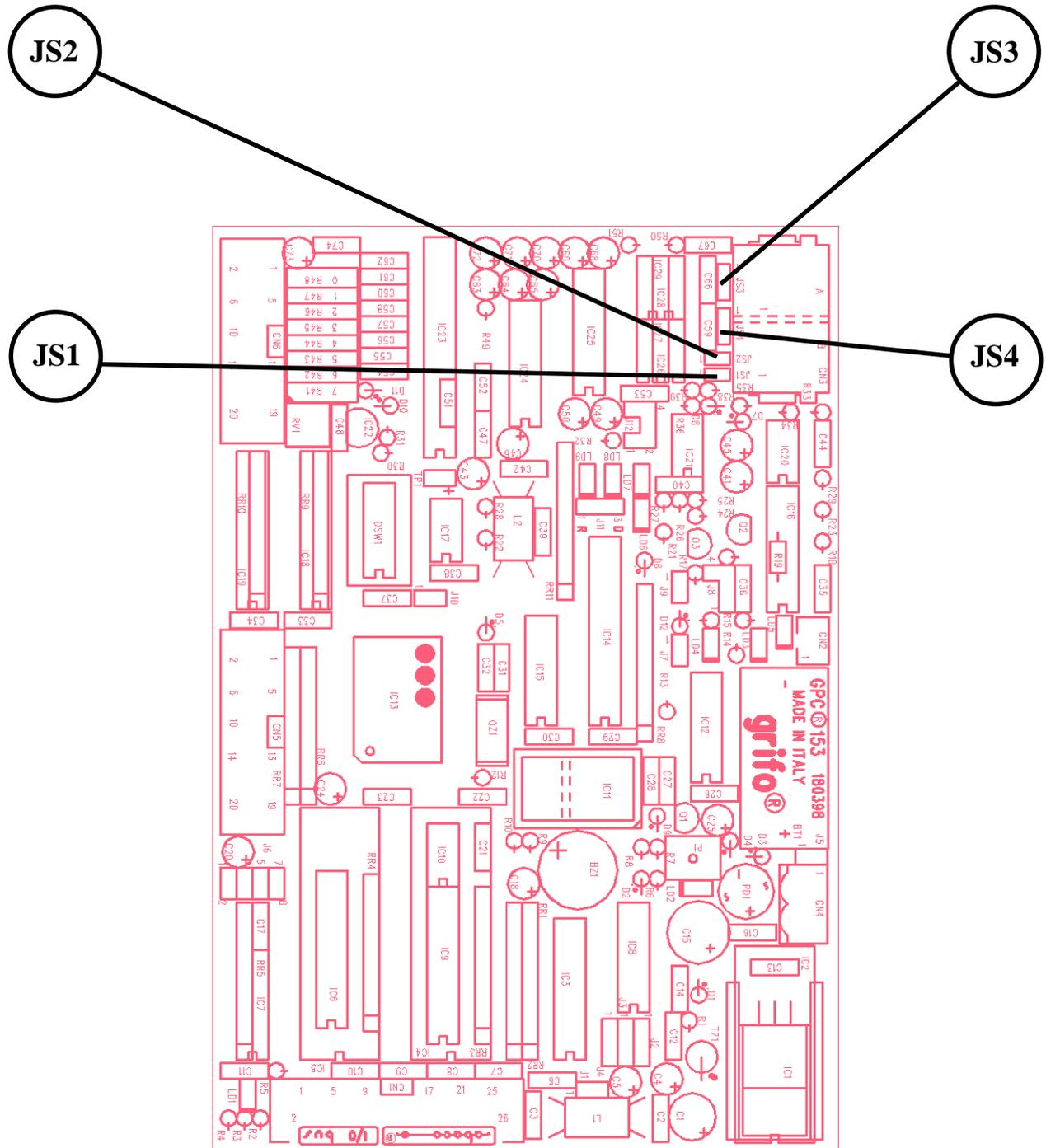
FIGURA 24: DISPOSIZIONE JUMPERS LATO SALDATURE
