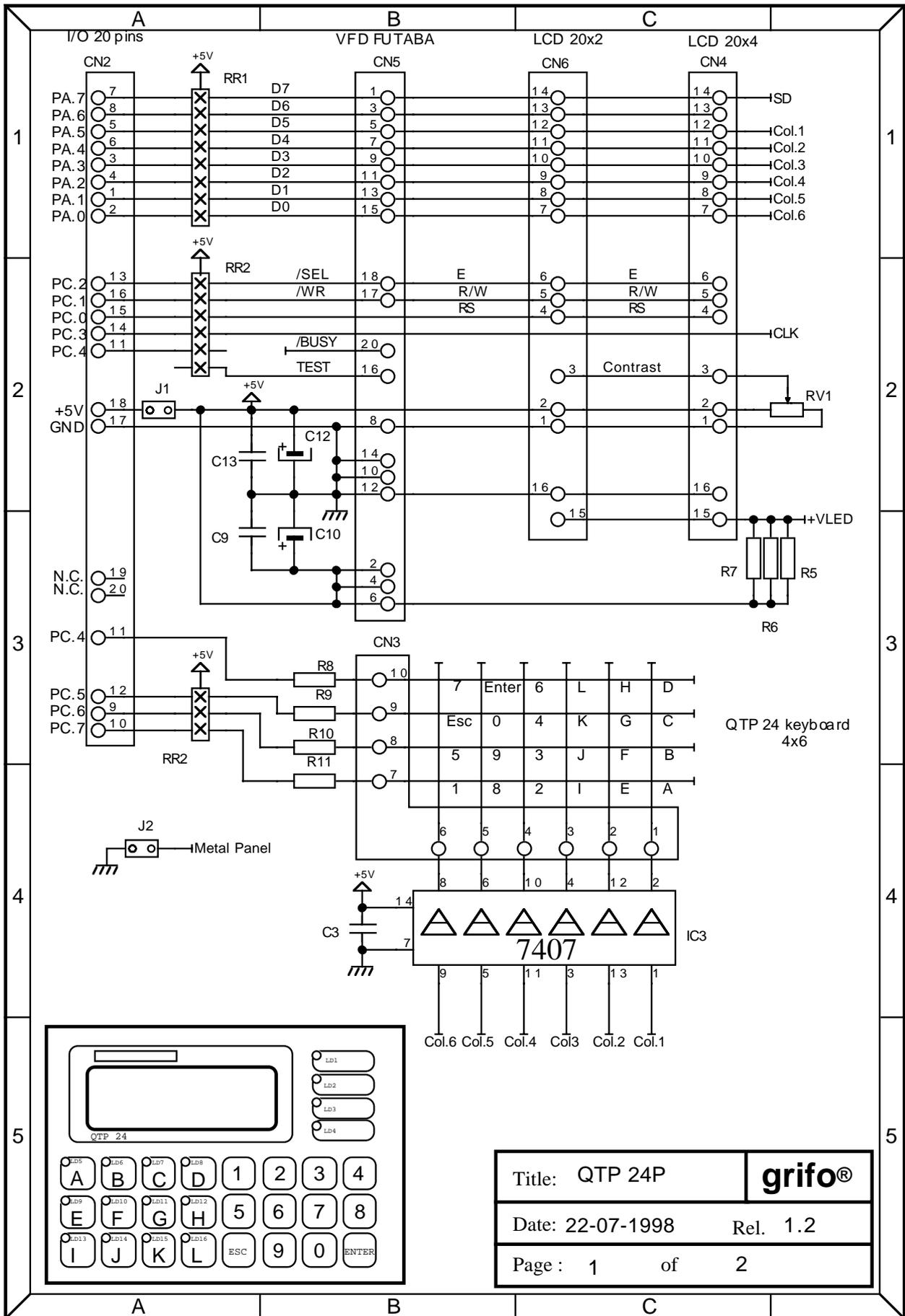
FIGURA A4: SCHEMA ELETTRICO QTP 24P - PARTE 1
