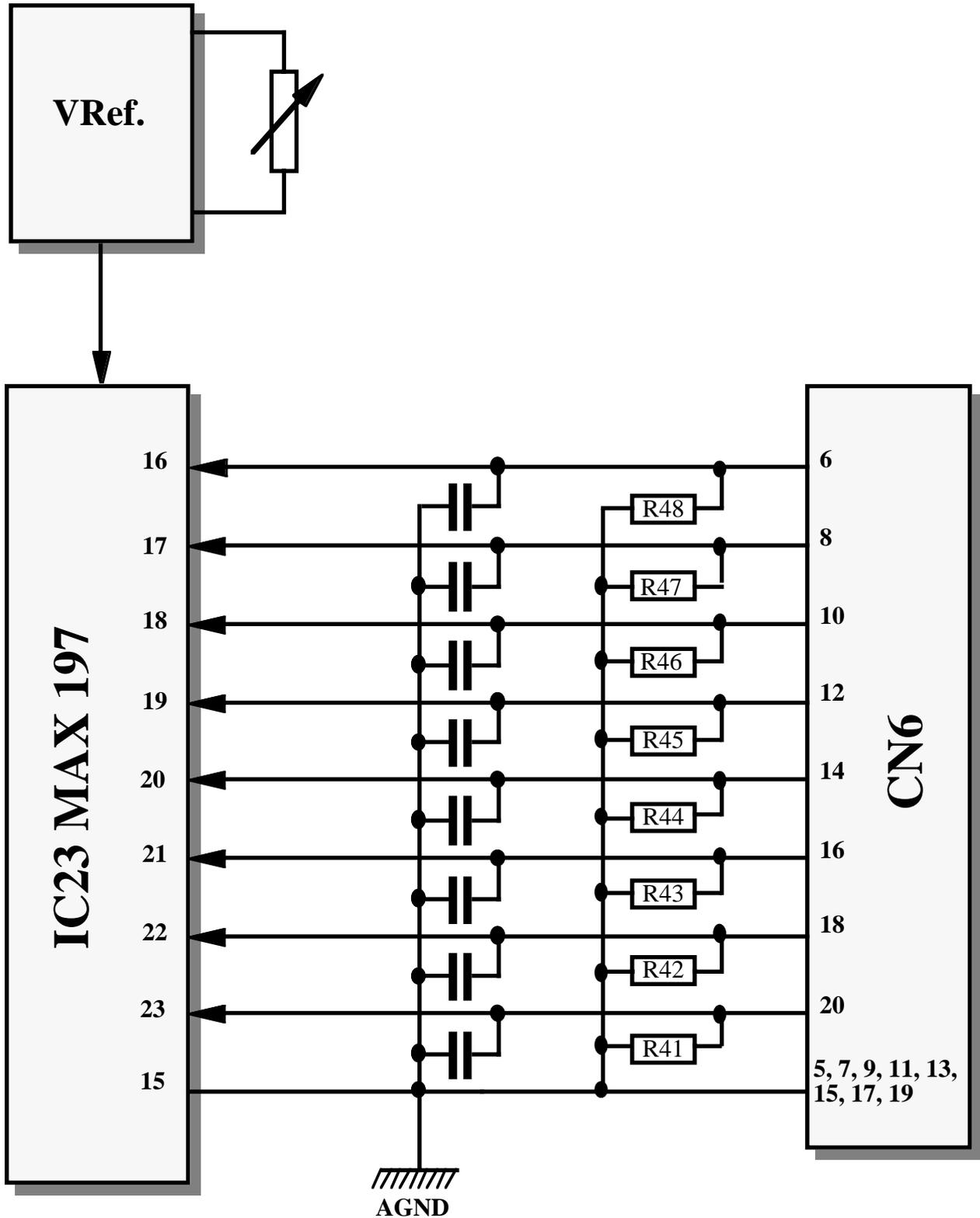
FIGURA 19: SCHEMA D'INGRESSO A/D CONVERTER
