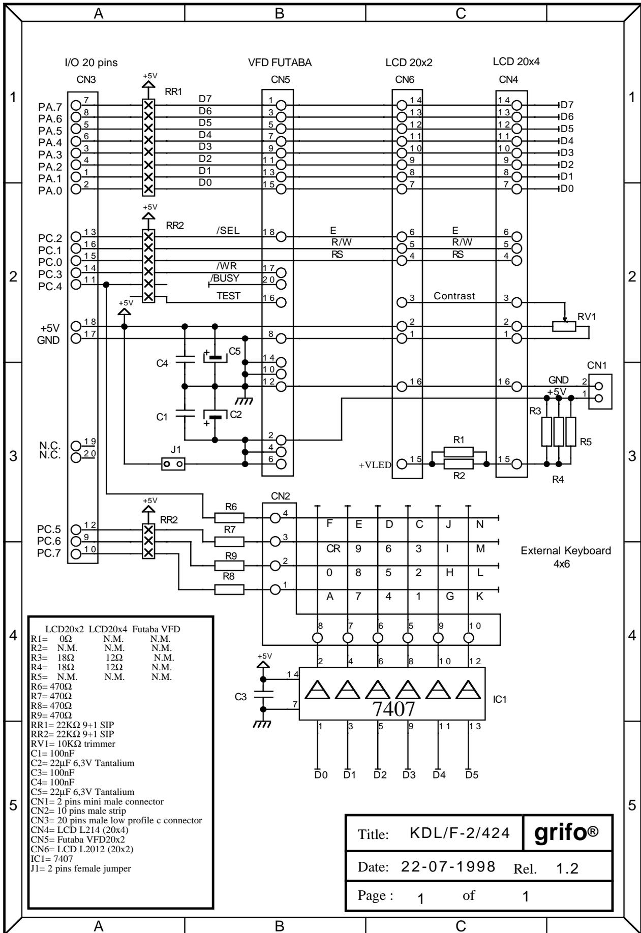
FIGURA A2: SCHEMA ELETTRICO KDX x24
