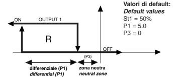
The diagram shows the functioning logic of the controller
