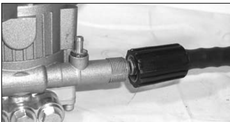
Figure 8 – Connect high pressure hose to pump
