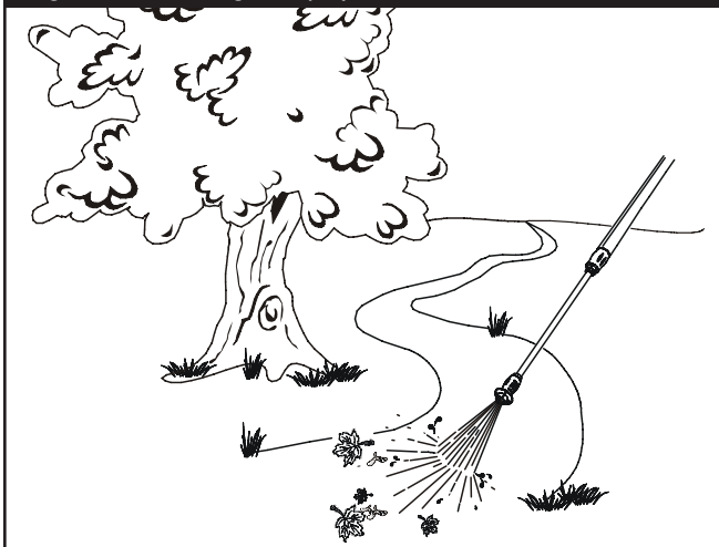
Figure 10 — Testing the Spray Pattern
