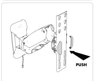
Step 8. Attach Mounting Rails To Display
