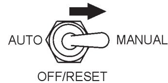
Figure 40. MPEC Control Switch (Manual Position)
