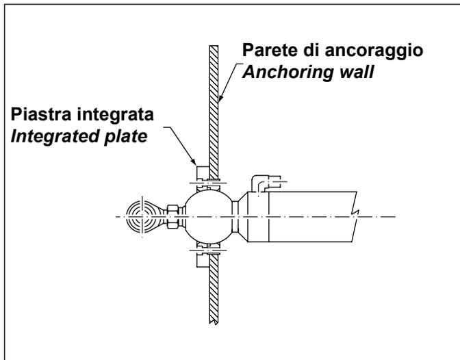
**Example showing how the cylinder may be anchored**
