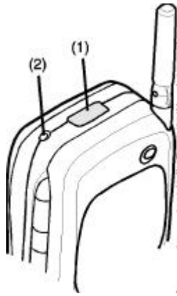
Figure 2-5: Ir port and antenna connector
