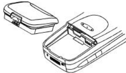
Figure 2-4: Inserting the battery
