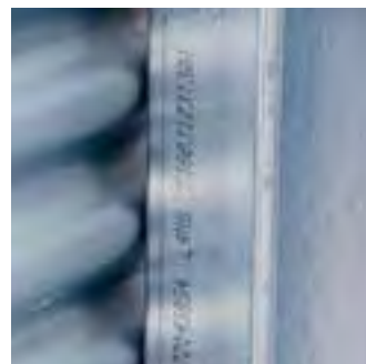
ENG. Every upright is marked on the back with the number of the coil from which it has been produced, the company identification code and the identification acronym
