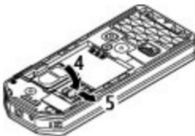
5. Insert the battery, and attach the back cover to the device.
