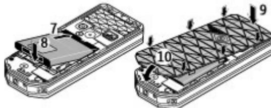
Observe the battery contacts (7), and insert the battery (8). Place the upper part of the back cover on the device (9), and close it (10).
