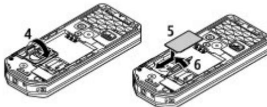
Open the SIM card holder (4). Insert the SIM card (5) with the contact surface facing down into the holder. Close the SIM card holder (6).
