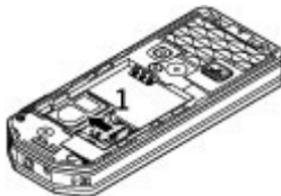
3. Open the card holder (2), and insert the memory card into the card holder with the contact surface facing inward (3).
