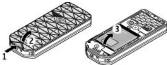
Slide the release button (1) to unlock and remove the back cover (2). Remove the battery as shown (3).
