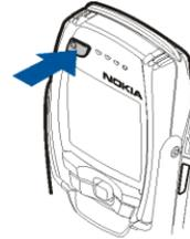
**TIPS ON EFFICIENT OPERATION:** Your phone has a built-in antenna. As with any other radio transmitting device, do not touch the antenna unnecessarily when the phone is switched on. Contact with the antenna affects call quality and may cause the phone to operate at a higher power level than otherwise needed. Not touching the antenna area during a phone call optimises the antenna performance and the talktime of your phone.
