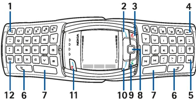
1. Keyboard light key
